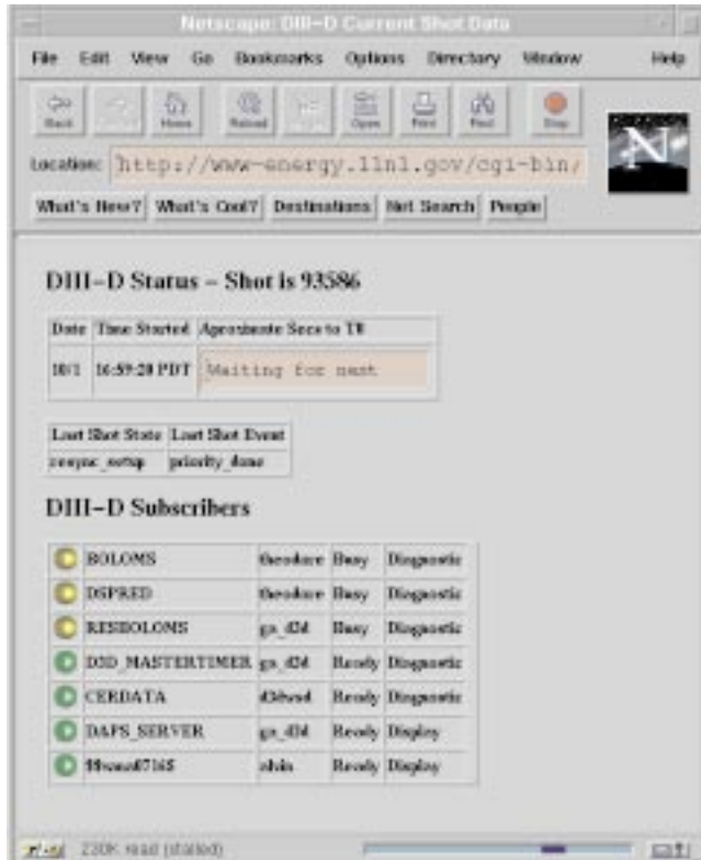
Figure 4. Status of instrumentation and experimental subsystems and state of the data-acquisition sequence, as displayed on a Web browser.
