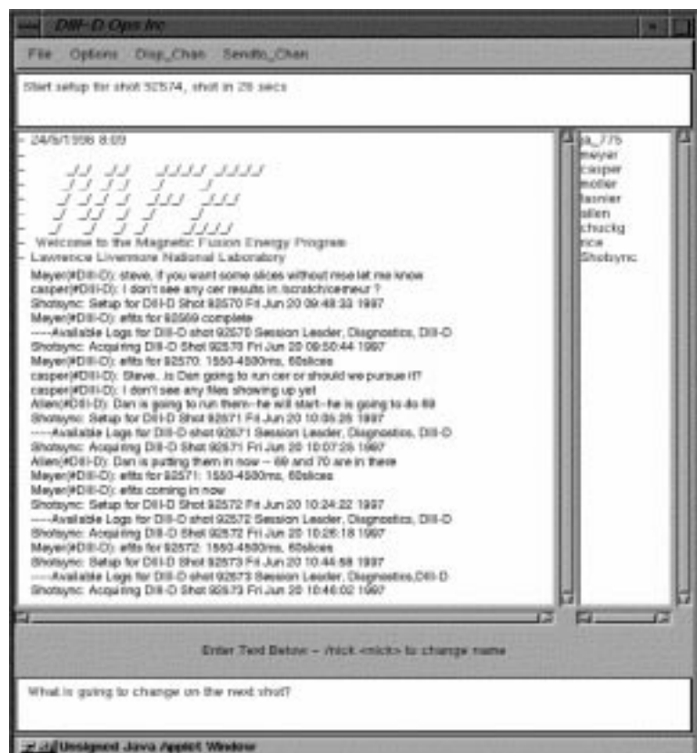
Figure 2. Java user interface to multiple-channel IRC-based communications showing countdown clock (top), dialog box (bottom), participants (right), and running history of dialog and operations (main box).
