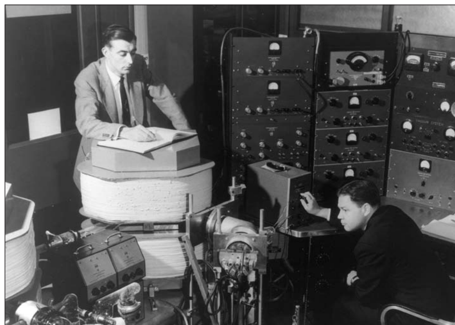
L–R: Timothy Collins and F.A. White operating a double magnet mass spectrometer used in discovering a new, naturally-occurring, radioactive isotope of tantalum, called Tantalum-180. The discovery of Tantalum-180 provided additional information important to the overall understanding of nuclear structure. The spectrometer, designed by F.A. White, is so sensitive that it achieves complete separation of isotopes even when one type may be more than a million times more plentiful than its neighbor. Credit: National Archives and Records Administration (NARA), courtesy AIP Emilio Segrè Visual Archives.
