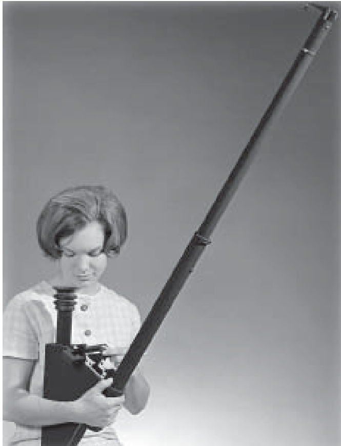
A visible skylight photometer, in the hands of Judy Steinacher for this 1967 photo. This portable version followed an earlier design from HAO veteran Jack Evans that was used in the 1940s to help identify appropriate sites to conduct research on the solar corona, including the Sacramento Peak Observatory at Sunspot, New Mexico. Courtesy of the University Corporation for Atmospheric Research.
