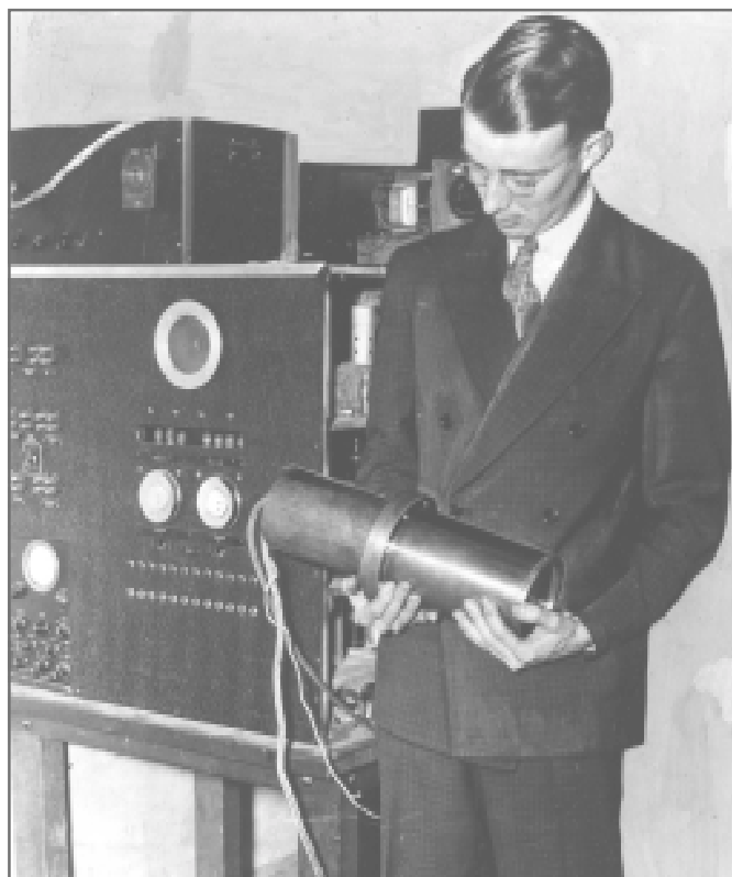
Luis Alvarez with personally built electronics and BF-3 ionization chamber, 1938. Donated by Peter Trower. University of California Lawrence Berkeley National Laboratory, courtesy AIP Emilio Segrè Visual Archives.
