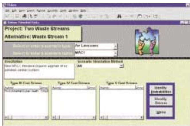
Figure 3. TCA's scenario builder combines probabilities and cost drivers for each scenario, allowing users to take into account high-dollar risks that may have a very small probability of occurring.
