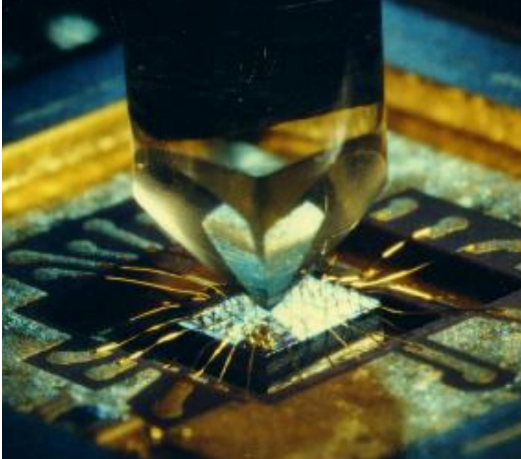
Figure 3. Electro-optic sampling combines ultrafast laser pulses and novel optoelectronic devices to generate and measure electrical pulses of the shortest possible durations.
