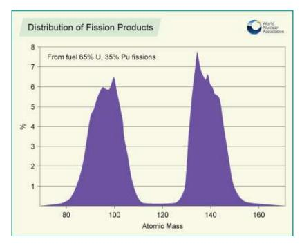
As you can see the distribution for Uranium and Plutonium fission products is bimodal with peaks around 95 amu and 135 amu. The most likely mass ratio of the products is 3:2 because it is the most energetically favorable. Here are two example reactions: <sup>7</sup>
