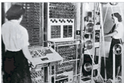
The original Colossus computer, 1943. Using vacuum tube and punched-paper-tape technology, operatives decoded German military messages during World War II. This artistic work created by the United Kingdom Government is in the public domain.
