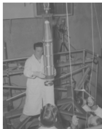
Explorer 1 satellite payload, technicians lowered the Explorer 1 satellite payload onto the launch vehicle's fourth stage motor. The photo was taken in the gantry at Launch Complex 26, Patrick Air Force Base, Florida, on January 20, 1958. Photo courtesy NASA/JPL-Caltech.
